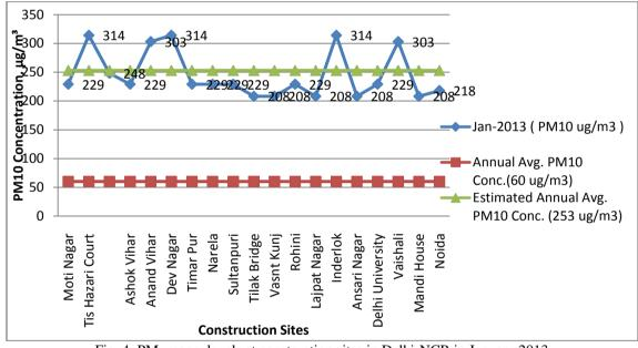
Fig. 4: PM<sub>10</sub> conc. levels at construction sites in Delhi-NCR in January 2013
