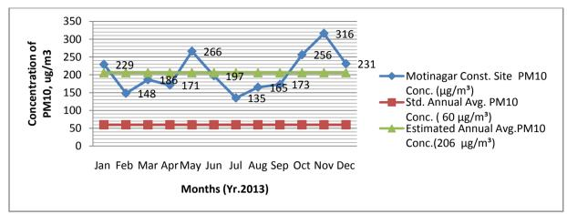
Fig. 2: PM<sub>10</sub> concentration levels at Motinagar construction site
